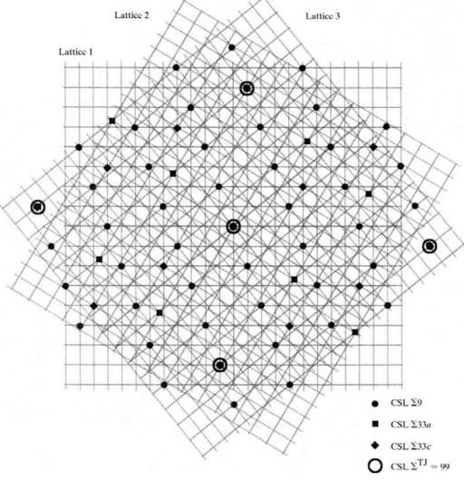
Figure 2 Superposition of three misoriented simple cubic lattices giving grain-boundary CSLs  $\Sigma 9$ ,  $\Sigma 33a$ ,  $\Sigma 33c$  and triple-junction CSL with  $\Sigma^{TJ} = 99$ . The projection direction is [110].
